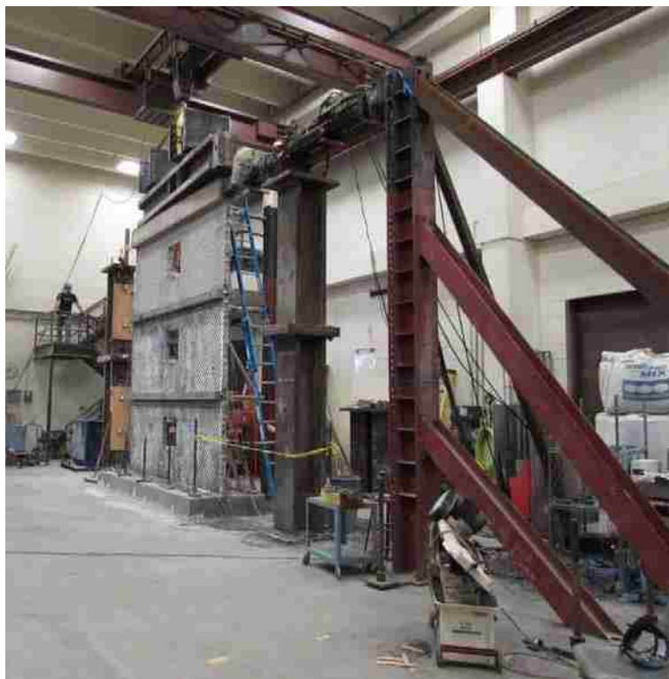
Figure 3-3: Reaction frame for testing
